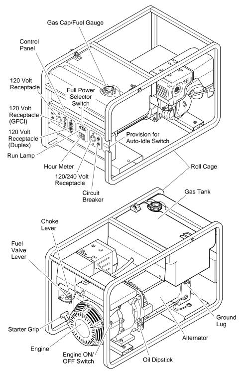
Figure 1 - Portable Generator (Model RGH5500A Shown)
